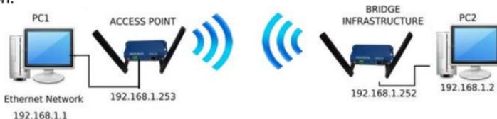
Set up the IP addresses according to the picture above and set the device connected to PC2 to Client (infrastructure) role.
