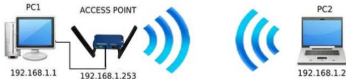
Set up the PC2 Wireless network interface according to the default parameters of the ACKSYS AP device (802.11gn, SSID "acksys", no security).
